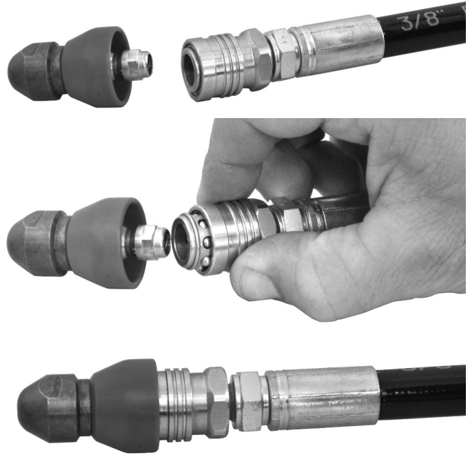
Figure.9 - Nozzle Quick Connect Operation
